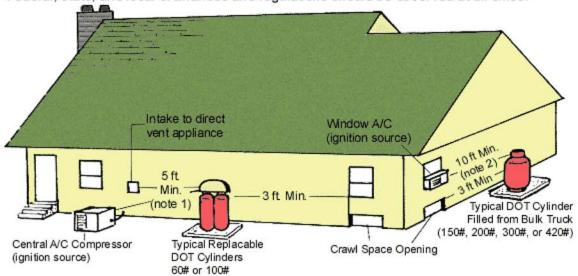
Notes: 1) 5 foot minimum between relief valve discharge and external source of ignition (air conditioner,) direct vent, or mechanical ventilation system (attic fan.)
